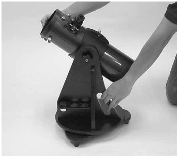
Figure 5. Try grasping the telescope as shown for easiest pointing. One hand moves the telescope from the front of the tube while the other hand remains on the handle to keep the telescope steady.
