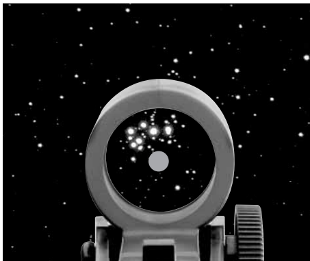
Figure 7. The EZ Finder II superimposes a tiny red dot on the sky, showing right where the telescope is pointed.
